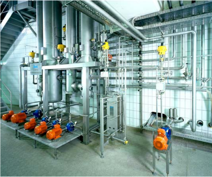
Bottom of the stripping column, condenser and heat exchanger from SIGMATEC
