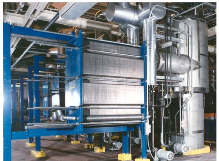
Five stage SIGMASTAR evaporator equipment with evaporation capacity of 18 m 3 /h
