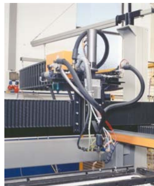
Robot-controlled gasket glueing assembly
