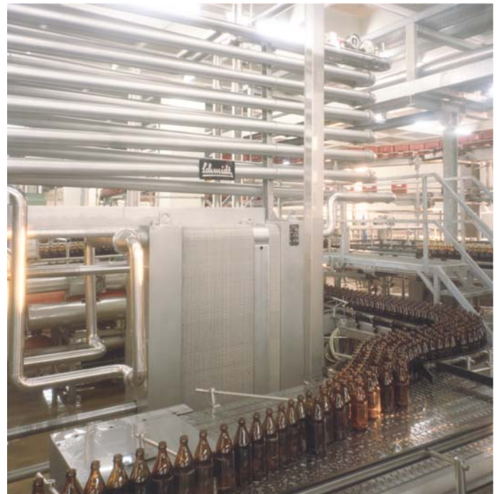
Short-time-heater for beer with SIGMA 66 plates, feed 325 hl/h
