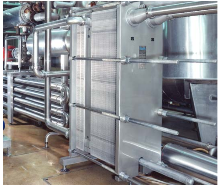
SIGMATHERM Short-time-heating system with SIGMA 66 for 300 hl/h wheat beer
