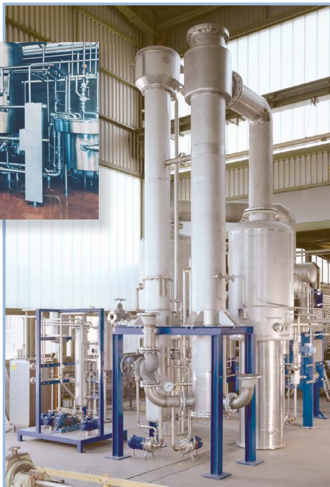
SIGMASTAR Concentration plant with aroma recovery
