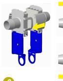
Align the connector halves with the pull tabs hanging down. Slide the two halves together. Independently squeeze each side of the connector until you hear an audible "CPC Click."
