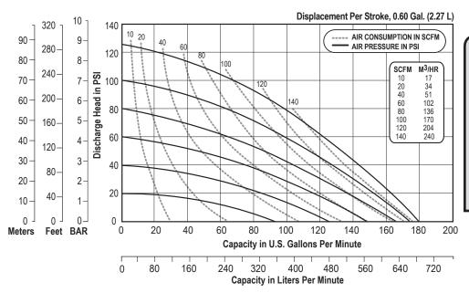
NOTE: Performance based on the following: TPE fitted pump, flooded suction, water at ambient conditions. The use of other materials and varying hydraulic conditions may result in deviations in excess of 5%.
