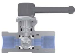
Valve open position
