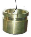
Lip seal location holds cocoa butter within pump Dove tail in bushing. Packing gland holds bushing in place. Used to pull bushing from pump
